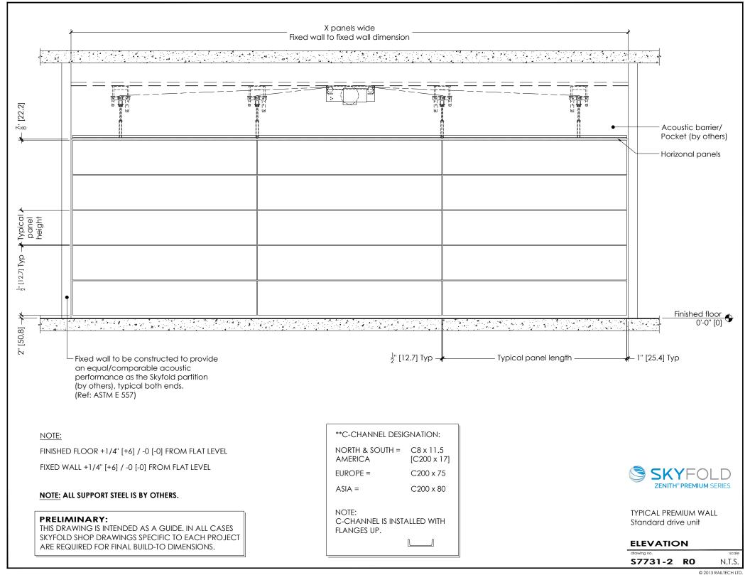
Standard motor unit & ceiling supports to be attached to C-channel\*\* before construction of acoustic barrier & pocket.
