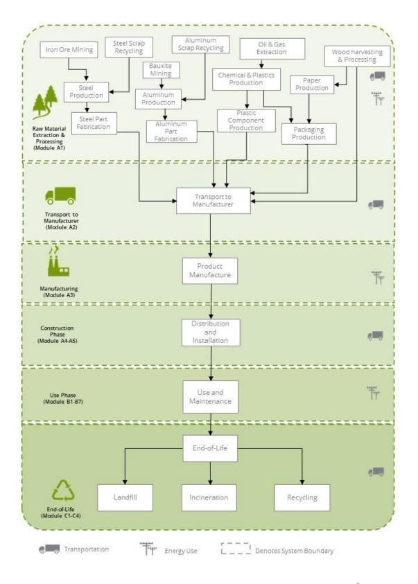
Figure 1. Flow diagram representing the major unit operations in the life cycle of the Skyfold Zenith<sup>®</sup> products.
