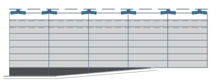
Vertical and horizontal panel joints are aligned with steps and other architectural features in the room.
